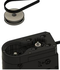
Then install the Belt and the 6oT pulley. Wiggling it a bit to fit the 2oT.
