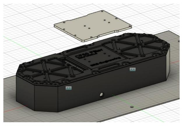
Fix the closing plate with M3x10 screws to ensure a good sealing.
