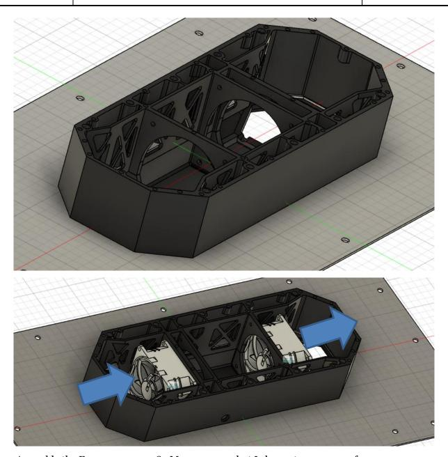
Assemble the Fan, you can use  $8x\ M3x50$  screws but I choose to use 10mm foam panner cutted the right length to pressfit them and dampening them way better
