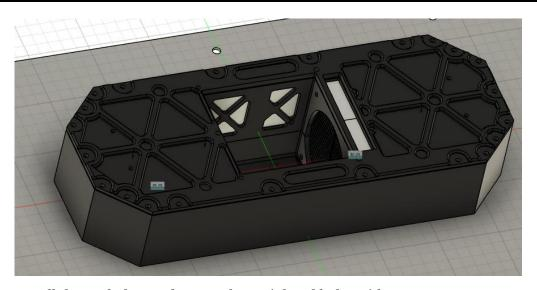
Install the Backplate and secure the peripheral holes with m3x10
