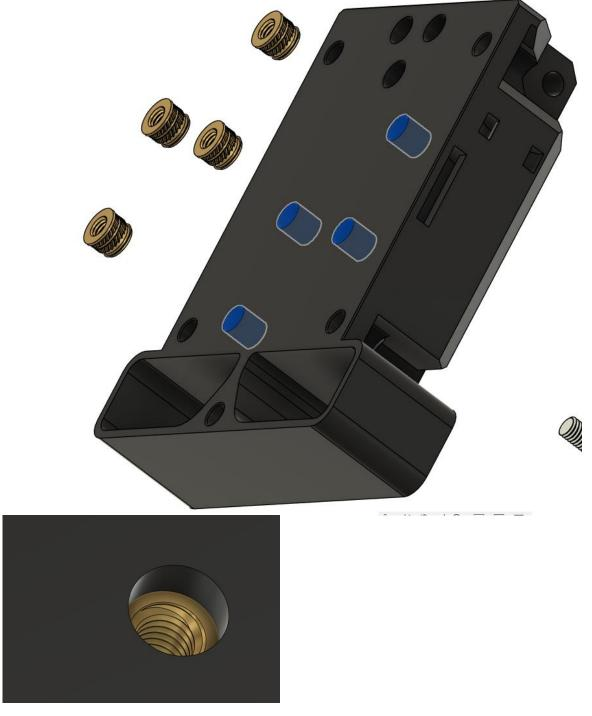
• Insert all heatinserts in the 4 holes, be sure to insert it further 2mm past the surface
