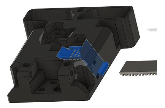
• Insert the belt in the orifice, push it to make the turn
