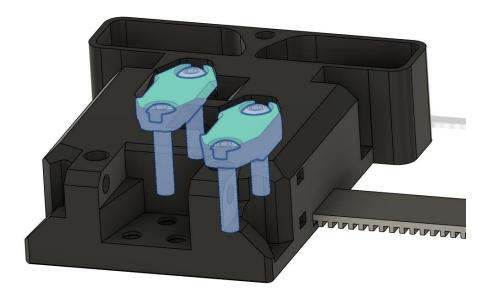
You can now secure the belts with the grabber with 2 M3x14 rounded head screws
