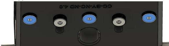
Then secure the ensemble with the x3 M6 countersunk the and 2x m5x15 screws at the top
