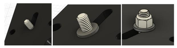
Install a m4 washer with a M4 nyloc nut on the other side to lock the mechanism.
