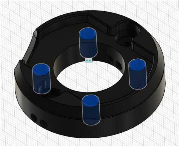
M4 inserts here on the lower ring
