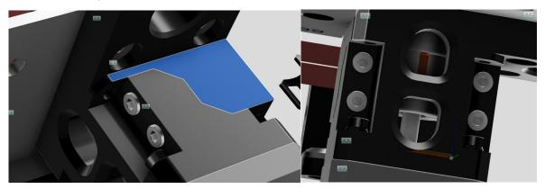
Try to screw or unscrew the 4 m3x30 screw to tune this coaxiality
