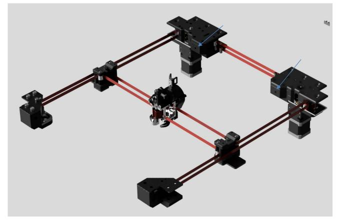
Apply the tension symetrically to keep an equilibrate tension, use the BRS Belt tensionning procedure (<u>https://github.com/FlorentBroise/BRS-Printers-</u>Mod/blob/main/manuals/belt.pdf)
