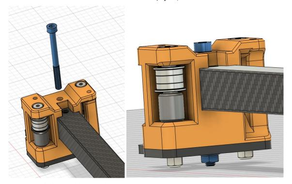
Secure the full assembly with the m5x45 screw
