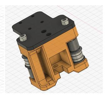
You can go for standard stock RR idlers, or the better solution of F695 bearings stacks (photos). Use the 2x 45mm shoulder bolts. Don't forget the 2 microshim m5x1mm on each side of each stack. Secure the bolt with the 2 m4 nyloc, no need to crush it!
