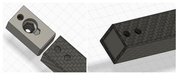
In order to completely secure the CF tube, this clamp goes inside each ends of the tube, to avoid crushings, and allow a very stiff assembly
