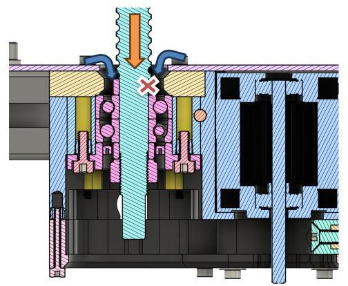
Assemble the ballscrew to the maximum, against the first spacer.
