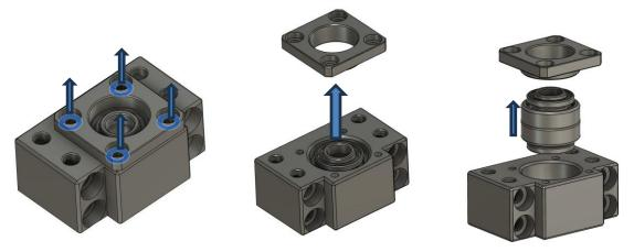
Remove the  $4x\,M4$  screws and remove carefully the internal, some force can be needed to remove the 608 bearings
