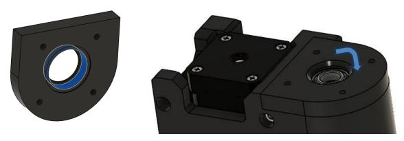
You can now place it on the M3 plate hole and add the 4x M3x45mm to retain it Don't forget to tight the anchors points (2x per blocks)
