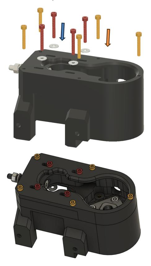
Add the retaining m4x20mm and m4x60mm bolts for the frame anchor. Add a M4 Tnut on each, Same logic for the rear part, but this time with a M4x90mm instead of the M6x60
