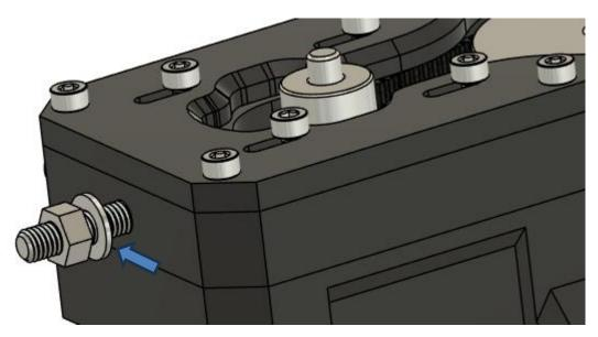
Now tune the belt tension through the M5 Nut + washer here
