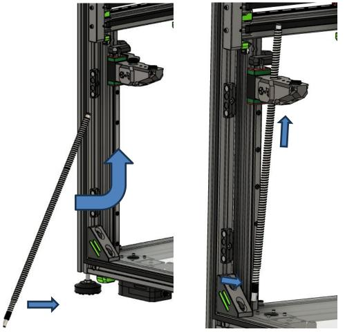
On this picture, the Nut and the Oldham are not represented, but should be positioned on the middle of the ballscrew BEFORE. **NEVER REVOVE THE NUT FROM THE SPINDLE**
