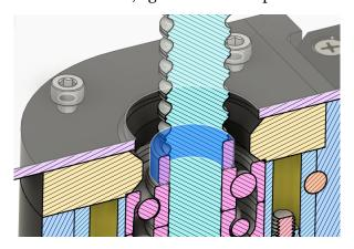
You need to first insert it in the arm hole, you may need to remove the top retainer to give you clearance, and then place the machined end in the lower motor block through the BK10 Internals
