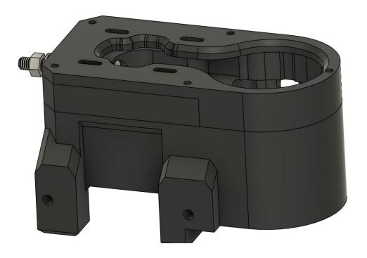
Then close it with the M3x22mm screw and then the M3x20mm to close the bottom. M3 washers are not mandatory.
