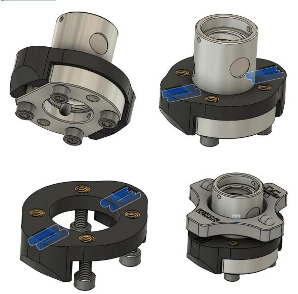
For the wobbleX (12/16), same logic: Ad some M5x20 to fix the BS nut to the lower ring, add the WobbleX middle ring and install it the same way with the spindle motion seen above.
