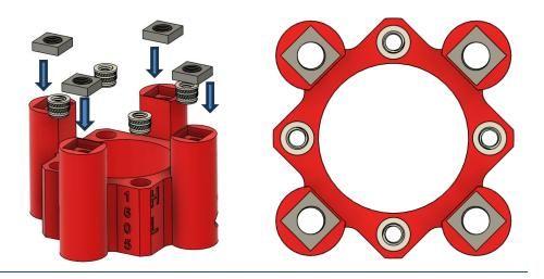
You need to pressfit with some Superglue points the Starlock design **WARNING: They** have a direction; ther is a notch on the side to align
