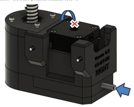
Push the M5 bolt to gain the minimal position.
