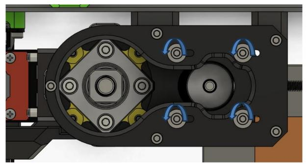
Unscrew a bit the 4 NEMA retainer screws
