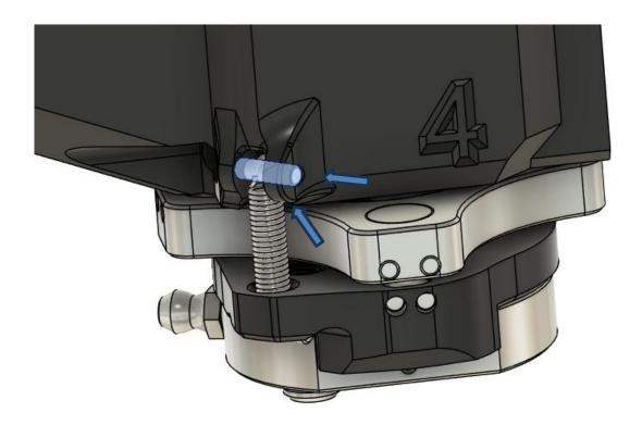
At the end of the unit assembly, use a plier to tension the spring and reach the arm mount point, secure it with a 3x6mm pin on each side
