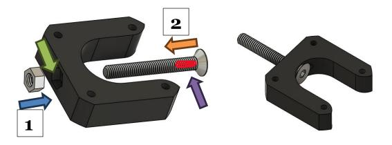
Apply glue in the nut part location. Install a M5 nut or a Nyloc M5, then let it dry 5 min. Apply glue on the first 6mm of the screw. Install the screw fully! Let it dry 10min
