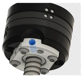
Apply grease un the nut, you can know if it's full by looking for grease presence under at the seal of the ballscrew, half a mm of it should appears. Close the hole with a grease nipple or a m6 headless 5mm screw
