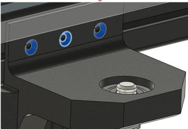
The rear retainer will serve as a support for the vertical 3030 posterior extrusion: remove the upper aluminium angle. The thin slide goes up on the upper horizontal extrusion, use the M3x14 screws with 3 m3 Tnut to secure it
