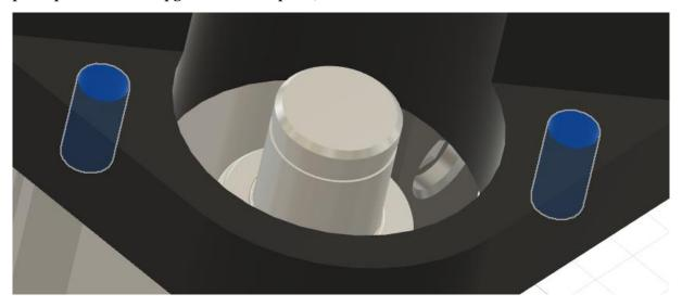
Then put 2 m2x8mm screw to fix the top part
