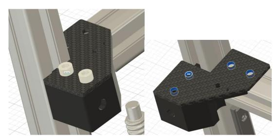
M6 screws are here to secure the plate to the part and the frame, put m6 washers for them
