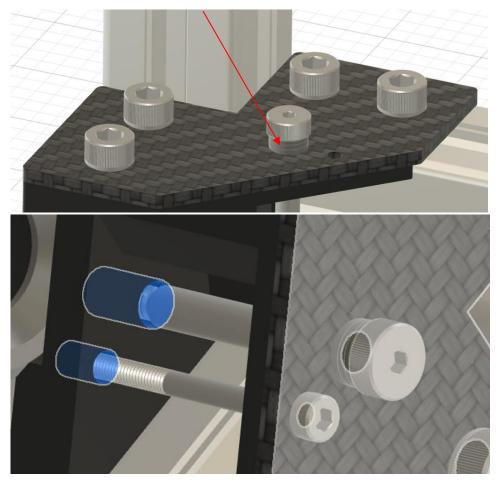
For the second RR plate assembly, use a nyloc m4 to secure the shoulder bold (don't put the shim)
