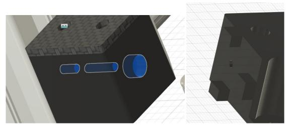
Don't forget the m3x40mm crew with the m3 t-nut to completely lock the part in place. You will see some notches that will match the 3030 profil to add stability and positionning
